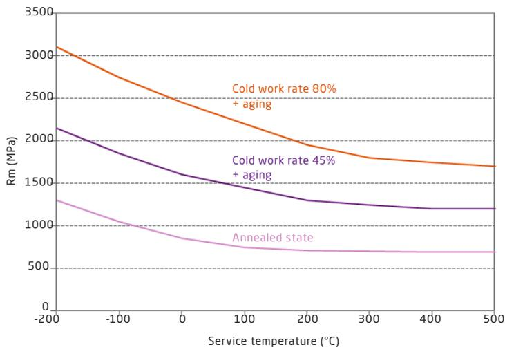
Figure 3: Influence of service temperature on ultimate tensile strength
