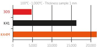
Our tests, carried out on V shape samples for  $100-1,000^{\circ}$ C, show that K44M exhibits good behaviour compared to austenitic 309 and to K41 grades.
