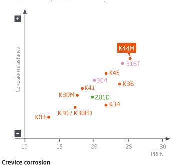
Due to the presence of molybdenum, our K44M grade has good resistance to the initiation of crevice corrosion, similar to that of our 316L austenitic grade. This resistance is measured in terms of depassivation pH. For K44M, this is in the order of 1.8, meaning it has minimal sensitivity to temperature.
