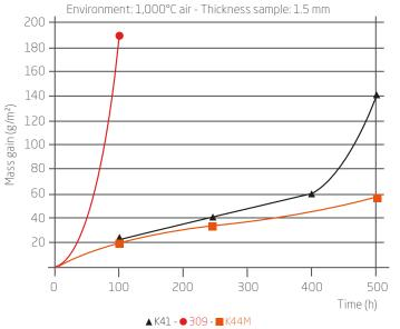
Compared to an austenitic matrix, the chromium diffusion in K44M's ferritic is easier. This avoids any loss in chromium and favours the formation of an oxidant protective layer rich in chromium.
