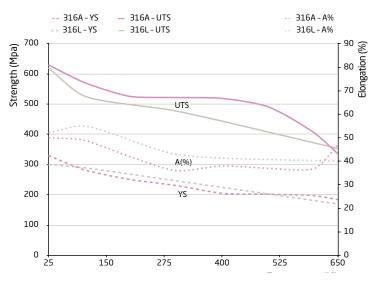
Method: 10 x 27 specimen. Preload = 30 MPa / Elastic rate = 0.5%·min·<sup>1</sup> Plastic rate = 2%·min·<sup>1</sup>.
