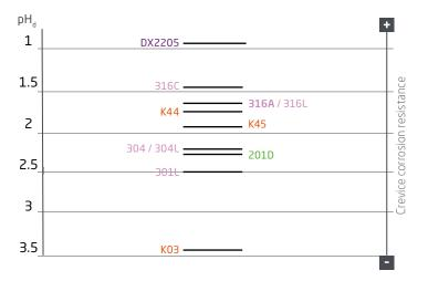
Crevice corrosion occurs in two stages. During the first stage (initiation), chloride accumulates and acidification begins. This eventually causes depassivation within the crevice region. A depassivation pH is the critical condition for passivity breakdown.
