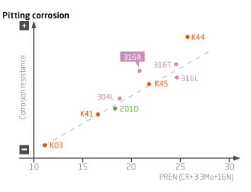
PREN based on composition does not reflect its real corrosion resistance.
