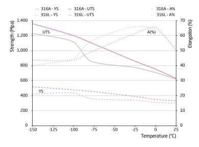
Method:  $10 \times 80$  specimen. Preload = 50 MPa / Elastic rate =  $8.8 \cdot 10^{.5} \cdot s^{.1}$ Plastic rate =  $6.47 \cdot 10^{.4} \cdot s^{.1}$ .
