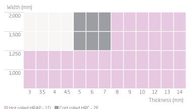
■ Hot rolled HRAP - 1D ■ Cold rolled HRC - 2E
