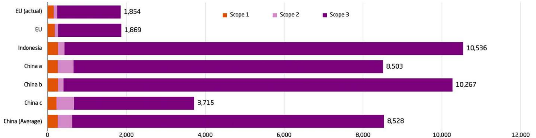
Actual and modelled carbon footprint for 1 t 304 black coil in EU, Indonesia and China (kg CO 2 -eq)
