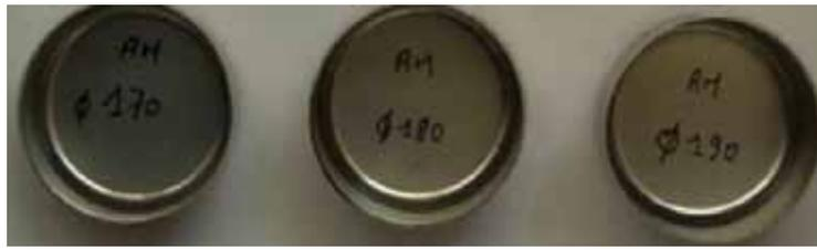
No delay cracking has been observed in air for drawing ratio up to 1.9.
