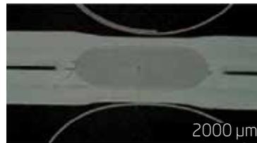
In resistance spot welding, there is no problem with homogeneous assembly, for example a joining of 2 x 1.5 mm with 450daN electrode force, a large latitude of current of 1.16 kA is achieved.
