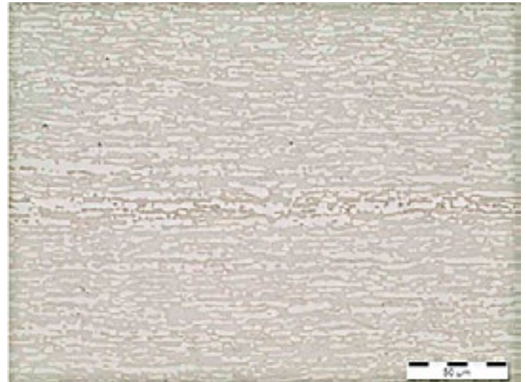
Example of the microstructure observed at mid thickness of the DX2507 (ferrite in grey, austenite in white) - no intermetallic phases detected.
