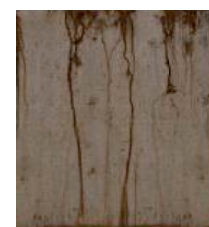
Aspect of K41X after exposure to road conditions Cycle duration: 24h Test duration: 500h Thermal treatment: 300°C
