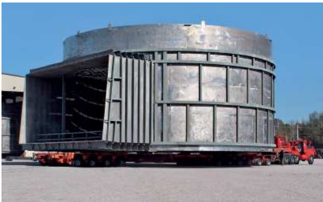
Flue gas desulfurization unit in 2205
