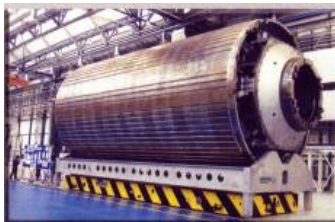
Mould for composite aircraft fuselage parts
