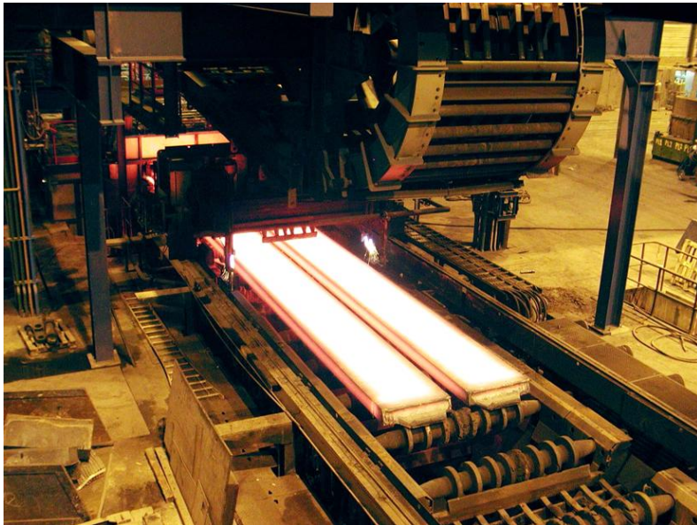
Steel Plant – casting up to 2m and twin casting
